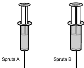
**Analysis of the assessment task- Answers and solutions:** To solve this task the student can use the relation between pressure, force and area,  $p=F/A$ . Neglect the hydrostatic pressure from the injection fluid. If the force that the staff applies to the syringe is the same, it is the area of the bottom that affects the pressure; the larger the area the less the pressure. The staff should choose syringe B.
